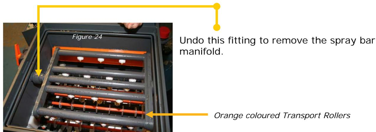
**NB:** to remove the bottom manifold, you need to lift out the transport rollers. (see figure 24).
