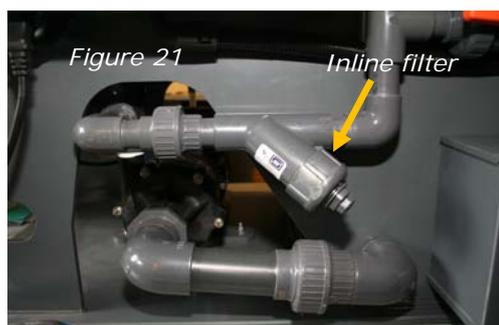
Remove the in-line filter (figures 21 & 22) ensuring you have some paper towels or a cloth underneath it to catch any drips.
