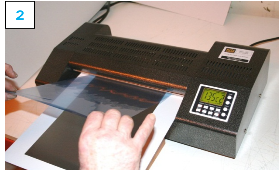
2. Laminate dry film photoresist to plate
