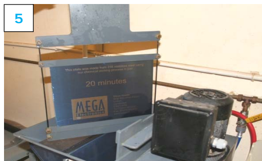
5. Alternatively spray develop in Mega Rota-Spray unit for finer detail
