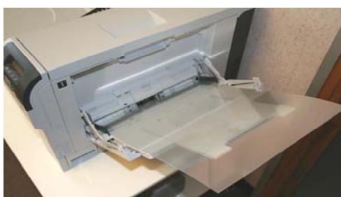
Load in bypass Tray
