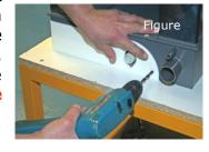
E) Remove Template and refit Drain Valve Handle
