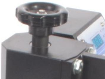
Set appropriate pressure using the Pressure Adjustment Knob, located on top of Heat Press.
