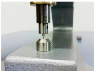
If upper and lower tool are perfectly aligned again, fix the brass cylinder with the headless screw again.
