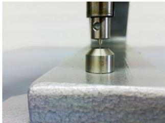
The Favorit undergoes strict quality checks before delivery. If it ever happens that the upper and lower tool of the Favorit is not aligned properly, there is a quick and easy way to recalibrate the tool.
