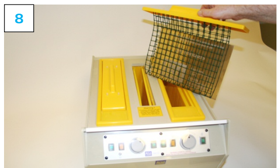
8. Strip off the photoresist in Mega Tri-Tank
