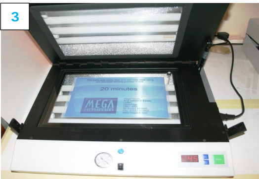
3. Expose image in Mega U.V. exposure unit
