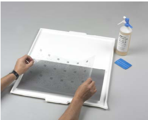
Laying the Laser Film
