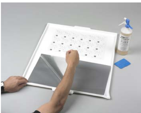
Peel off liner from Base Sheet
