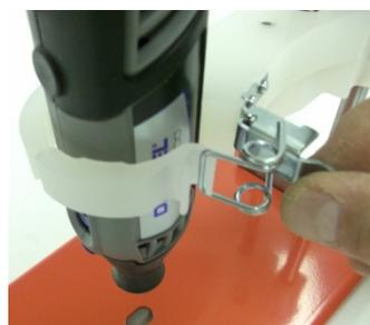
**Note:** If your drill is too small you may need to pad the clamp out with a soft material or make some sort of adaptor. If your drill is too large, then you may have to source some assistance from a local engineering company to machine some material off the contact areas in the clamp.
