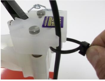
5) Push the cable of the drill into the slot in the pillar head and lock in place with the cable tie. The cable tie is releasable/reusable, so it can be unfastened to remove the drill.
