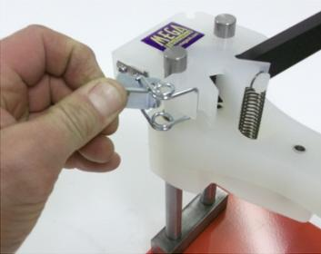
6) When the drill bit is fitted in the drill it may be necessary to adjust the height of the drill assembly, as you only need approximately 5-7mm clearance between the drill tip and the PCB material.
